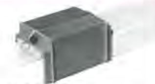
Transfer end (fitted) — Ref. TE 16 140 (Trolley-collector enters from 1 track into a contiguous or switching track. Alignment plus/minus 3 mm. Gap 2 to 10 mm between 2 Transfer-ends.
