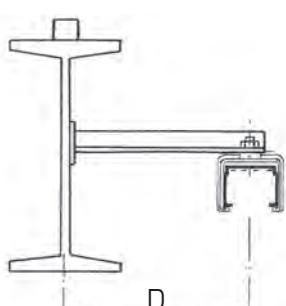
Suspension by support welded
